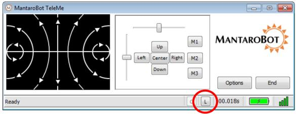
If the MantaroBot is equipped with a Laser Pointer the "L" button at the bottom of the Controller window will not be grayed out. Clicking on the "L" with your mouse or alternatively hitting the "L" button on your keyboard will turn the laser on/off. The laser can be pointed by using the Camera Control functions and turning it on while the camera is facing the location of interest.
