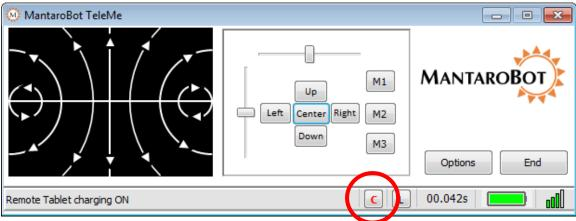
During a call, there may be instances when the internal battery of the TeleMe has plenty of charge but a person local to the TeleMe may notice that the user device plugged into the device holder is running low on charge. In those instances, the remote user has the option to charge the user device (only while the
